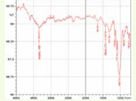
FTIR spectrum of desized cotton sample using NIB alpha amylase
